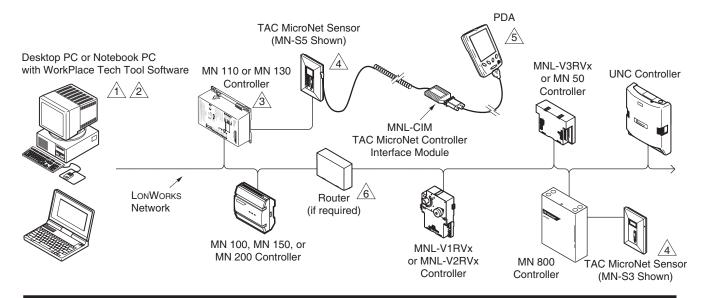
A PC can be connected to the LonWorks TP/FT-10 Network, either directly or through the LonWorks® network jack of a LONWORKS controller or MN-Sxxx Wall Sensor. The PC must have an Echelon® LonTalk® adapter card.
