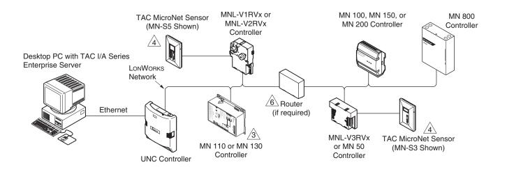
Figure-1 TAC I/A Series MicroNet MN VAV Series Controller Connectivity.
