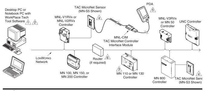
A PC can be connected to the LonWorks TP/FT-10 Network, either directly or through the LonWorks network jack of a LonWorks controller or MN-Sxxx Wall Sensor. The PC must have an Echelon<sup>®</sup> LonTalk<sup>®</sup> adapter card.
